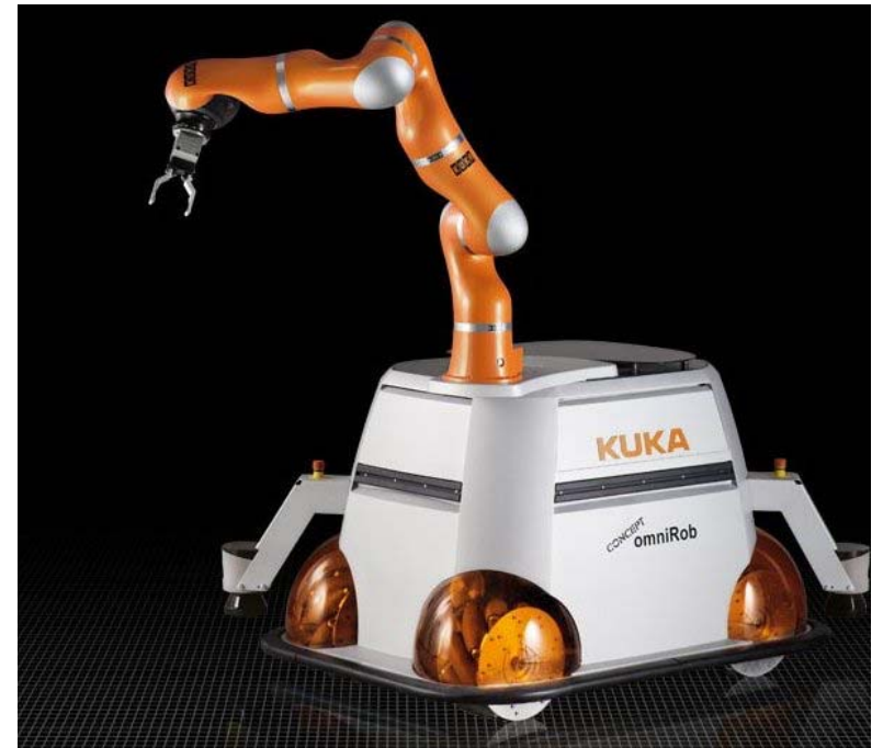
Kuka iiwa max 14 kg (175 platform) mass= 375kg
